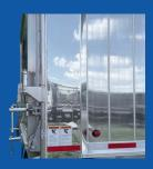
top pin is hidden and protected inside the rear post. The Side Swing Tailgate Guide Ramp Roller prevents top pin misalignment by guiding the gate and top pin back into position during closing, making the gate much easier and faster to close.
