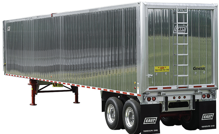
Enviro Recyclers Inc. uses East Genesis smooth-sided aluminum refuse trailers like this one to haul trash and recycling.
